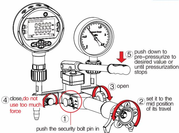
**D** *Pressurizing process and fine adjustment*
